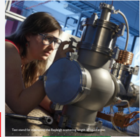
Test stand for measuring the Rayleigh scattering length @GSI-Linac
