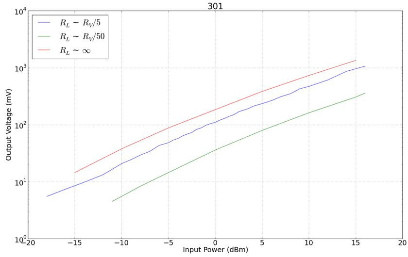
Figure 2: Output voltage vs. input power for the 301S diode.
