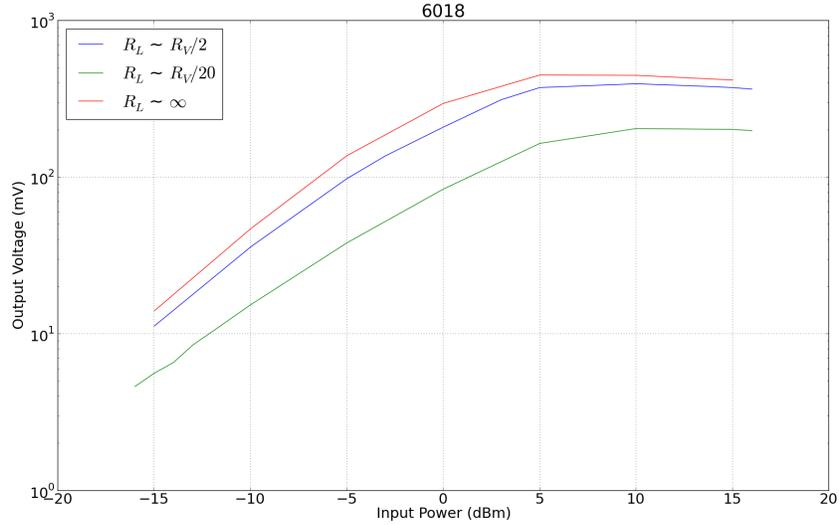
Figure 3: Output voltage vs. input power for the KDT6018 diode.
