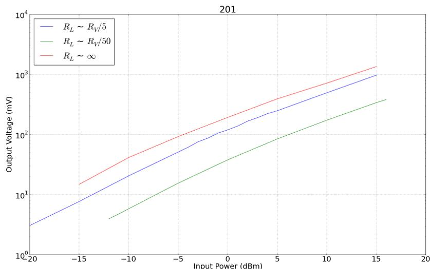
Figure 1: Output voltage vs. input power for the 201S diode.
