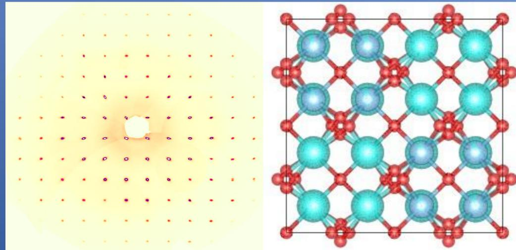
Figure 2: A projection across the  $hk0$  plane (left). The discoloration around the central peaks is due to variation in absorption. The right displays a side on view of the structure of the crystal.
