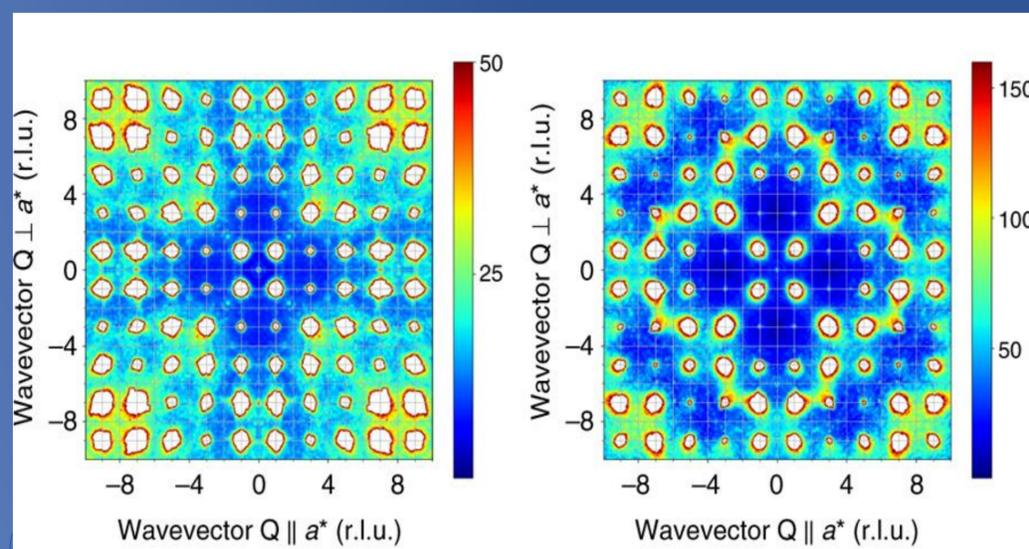
Figure 1: Results from Bowman et al [1]. These are two neutron scattering patterns for an Oxygen depleted (left) and stuffed form (right) of Ytterbium titanate.
