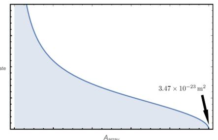
Parameter space for 'cooper pair box' regime of qubit operation. The maximum allowable value of the array area is the x-intercept, taking a value of  $3.47 \times 10^{-23} \text{ m}^2$ , which would mean an aperture width of  $\sim 6 \times 10^{-12} \text{ m}$ , or 5% of the width of a helium atom.
