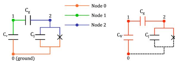
$$\mathcal{L} = \frac{C_v \dot{\Phi}_1^2}{2} + \frac{C_g}{2} (\dot{\Phi}_2 - \dot{\Phi}_1)^2 + \frac{C_J \dot{\Phi}_2^2}{2} + E_J \cos\left(\frac{\Phi_2}{\hbar}\right)$$
