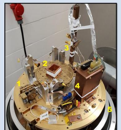
Internals of the cryostat. 1.) Probe that 'pinches' to take measurements from the isolated stage 2.) Isolated stage which is cooled below 1K to which the sample is attached 3.) Rigging to suspend the sample and solenoid 4.) Internal circuitry that enables measurements 5.) Thermally isolated layers which are each at a lower temperature progressively inwards
