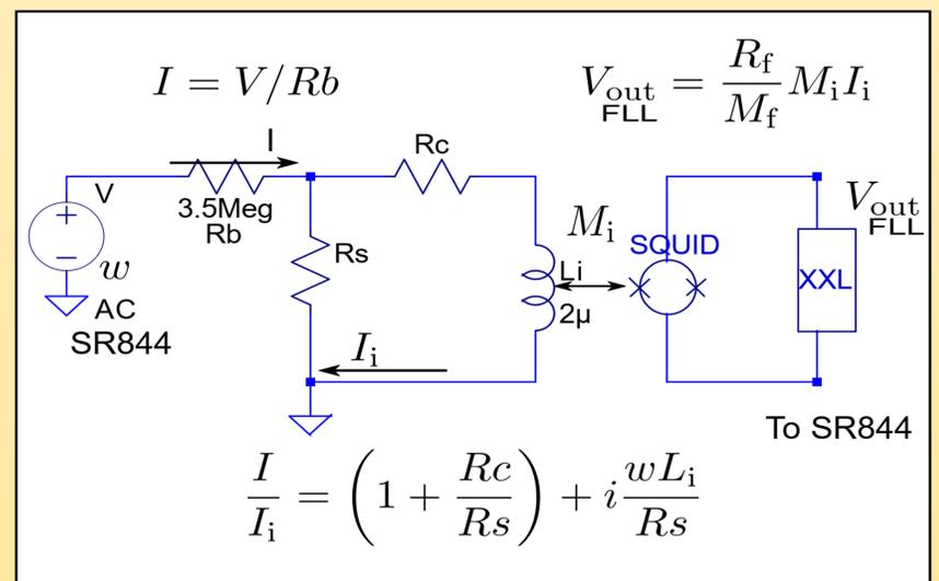
Figure 2: Proposed SQUID-based resistance measurement scheme. The SQUID is operated in flux-locked loop (FLL) mode. The voltage output,  $V_{\text{out, FLL}}$  is proportional to the current in the input coil,  $I_i$ . The bias current,  $I$  is of the order of  $\mu\text{A}$  due to the  $3.5 \text{ M}\Omega$  shunt resistor.
