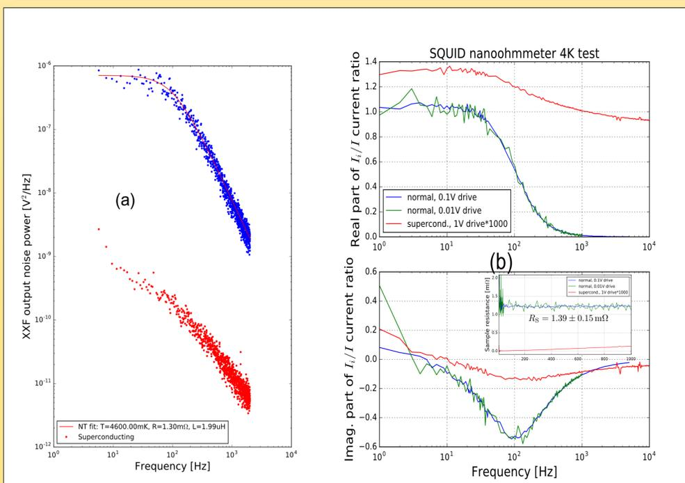
Figure 3: Resistance measurement of the tantalum sample using two different schemes: (a) SQUID Johnson noise measurement (b) SQUID-based conventional transport measurement (SQUID Nanoohmmeter). The measurement output when the sample is normal is compared to the superconducting case. They show excellent agreement to the theory.
